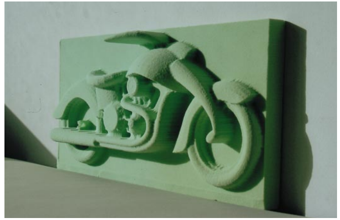
Figure 5: A CNC milled concept model in foam of the geometry shown in Figure 4 (courtesy of Delft University of Technology and Sonny Lim)
