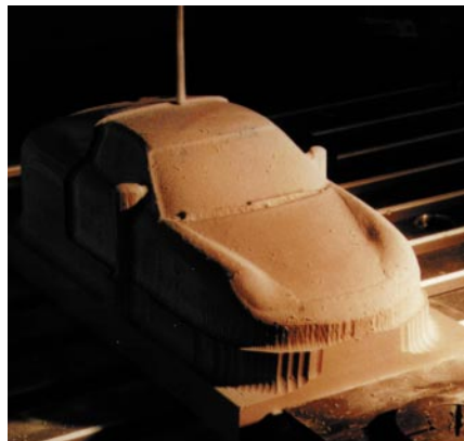
Figure 9: Milling the top of a scale model Porsche in tooling board. After first roughing, the actual surface is milled
