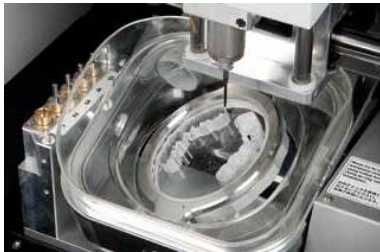
5-Axis machine 1 (Roland DWX-50, for dental applications).
