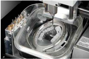
5-Axis machine 1 (Roland DWX-50, for dental applications).
