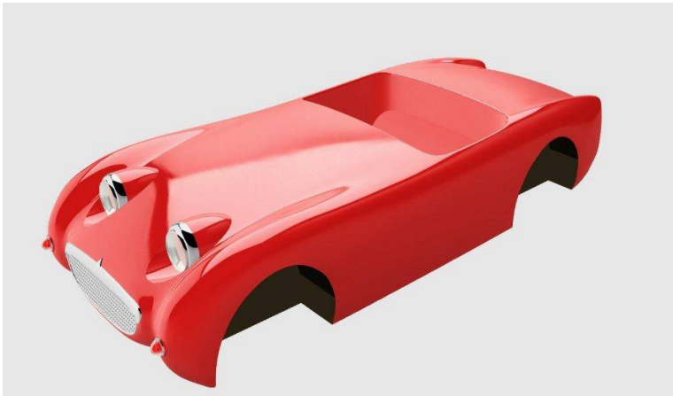
The car body geometry in CAD.
